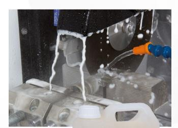
*To control the correct fluid dosage use the REFRACTOMETER Code 60 CT900 10*
