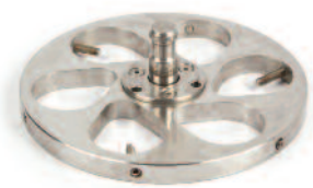
Stainless steel sample holder for central pressure
